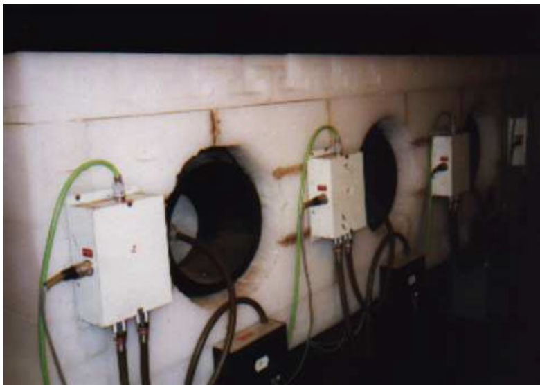
Fig.2. The detail of the neutron monitor placed in the small measurement building on the roof of the main one at Lomnický Štít. There are used 8 proportional counters of the type SNM-15.
