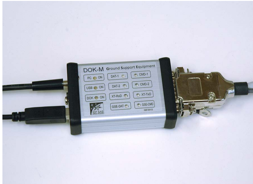
Figure 18. Ground Support Equipment of DOK-M (without external power supply).
