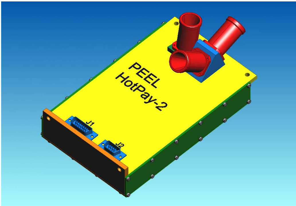
Figure 2-2. The PEEL instrument – virtual 3D model
