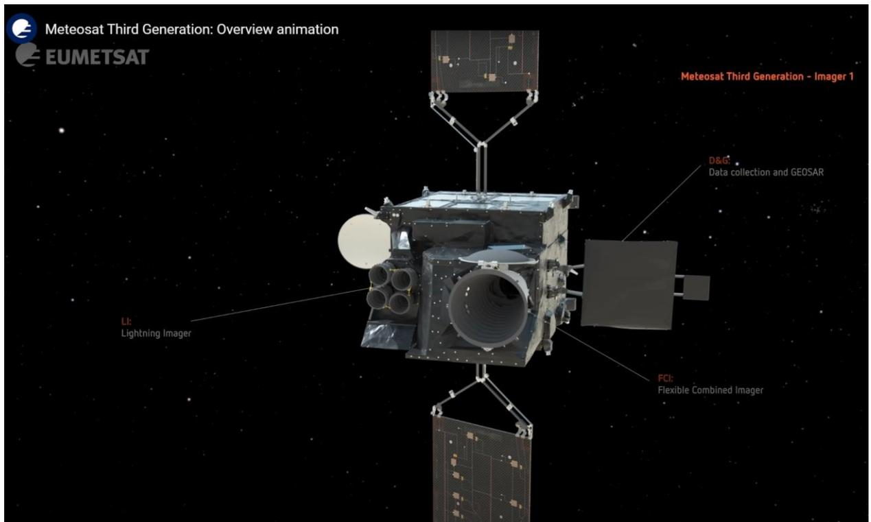
**Figure 6.1.** MTG-1I satellite and its instruments.
