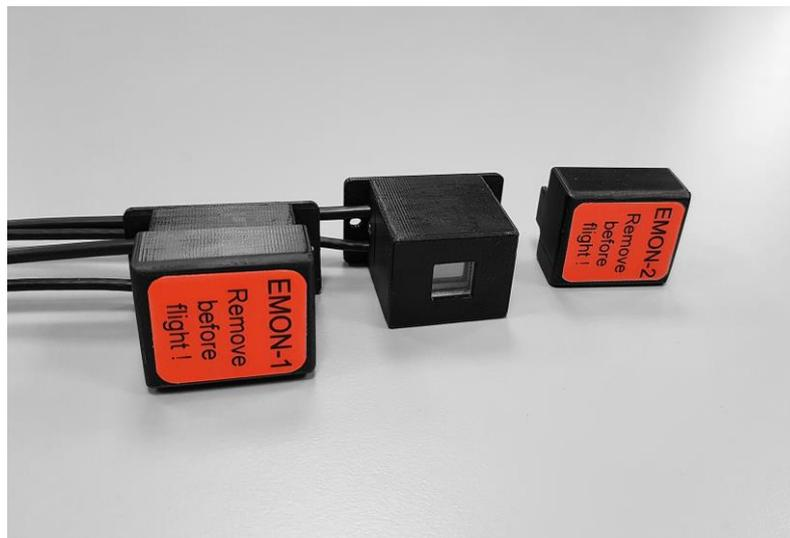
*Figure 1.7. A pair of the EMON photo-detectors developed at IEP SAS for NASA-SPB2 mission.*
