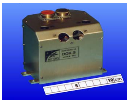
Fig.7. The detector block of DOKS, the simplified version of DOK2, for medium energy particle measurements at Magion 5 developed at IEP SAS Košice with the Technical University of Košice.
