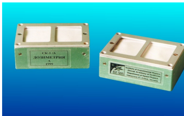
Figure 5.6: The stacks of passive detectors of CRs exposed on MIR station during the mission of the Slovak astronaut I. Bella in February 1999.
